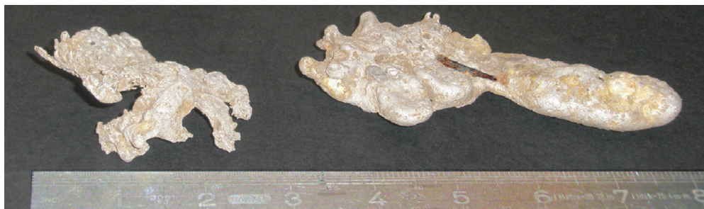
Two pieces of aluminium – or Duralumin alloy – found off Tanner's Lane. Left: a thin wafer probably from the 'skin' of the Spitfire. Right: a much thicker piece, about 5 inches long, melted in the intense heat of the post-crash burning of the Spitfire's aviation fuel. In its middle is a rusted steel rod, around which Duralumin was rolled to strengthen curved opening parts, such as the engine cover
